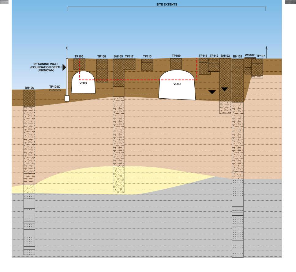
The basement was overlaid onto these cross sections showing that the proposals do **not reduce the thickness of the underlying Boulder Clay**.
