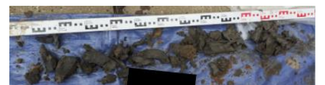
Fig 4. Hand auger arisings from HP3 (1.2-2.1m depth). Elevated PID readings and a strong hydrocarbon odour were recorded between 1.4-1.7m depth.
