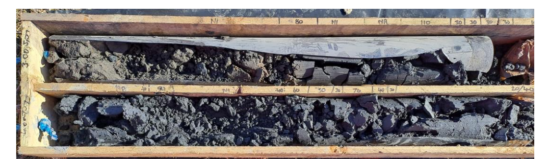
Fig 3. Photograph of drill arisings showing a change in soil colour, the threshold at which less impacted brownish grey ash sediment above (10mAOD) separates highly impacted blueish grey ash sediment below (9mAOD).
