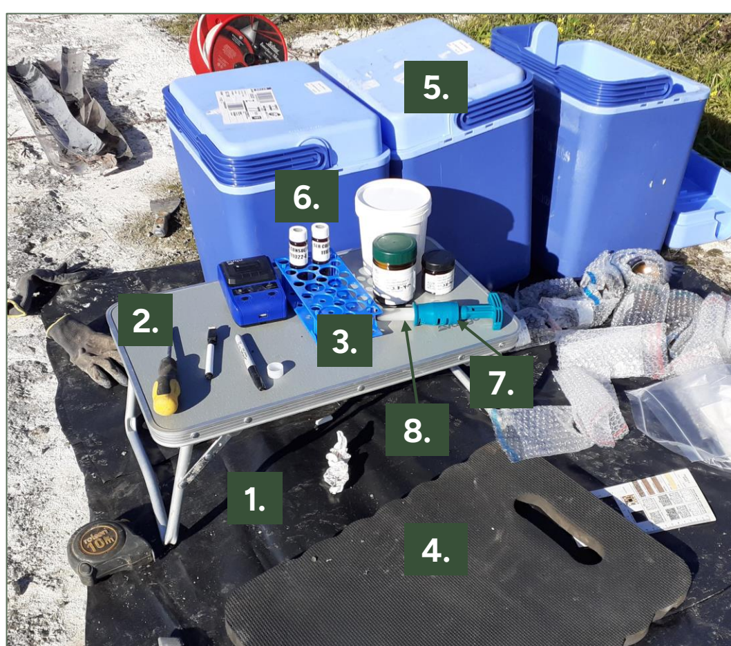
Fig 1. Field application of BS10176 soil sampling method using methanol preservation.
