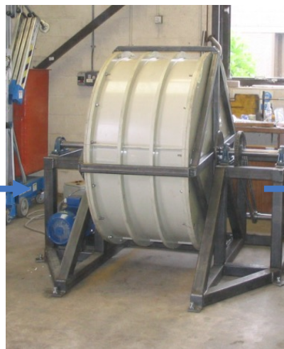
Sample is homogenised in the mixing drum for 10 days
