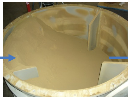
Crushed and dried sample is loaded into the mixing drum
