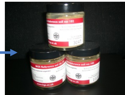
Homogenised sample is split into 50 g batches prior to homogeneity testing and certification
